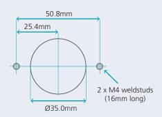
Pushbuttons with Compact 3 and Compact 3P switch bodies can be supplied loose or incorporated into stations. These have a vertical pitch of 50mm and a horizontal pitch of 60mm (Compact 3), or 80mm (Compact 3P), which means the switch body can be rotated 90 degrees.
