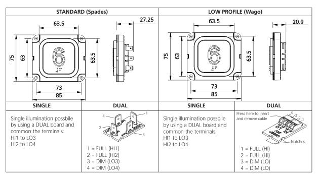
Please note the orientation of PCB notches to the tab (Stanard) or Wago connector (low profile) numbers
