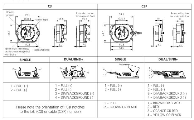
Compact 3/3P Pushbuttons can be supplied loose or incorporated into stations with 1.5mm or 2.5mm stainless steel faceplates, with a vertical pitch of 50mm and horizontal pitch of 60mm (C3) or 80mm (C3P) i.e the pushbutton body can be rotated through 90 degrees (horizontal version shown above). If pushbuttons are supplied loose, spacers are provided to accommodate the differing faceplate thickness.
