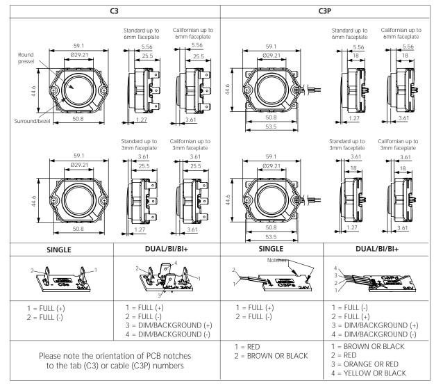
Compact 3/3P Pushbuttons can be supplied loose or incorporated into stations with 1.5mm or 2.5mm stainless steel faceplates, with a vertical pitch of 50mm and horizontal pitch of 60mm (C3) or 80mm (C3P) i.e the pushbutton body can be rotated through 90 degrees (horizontal version shown above). If pushbuttons are supplied loose, spacers are provided to accommodate the differing faceplate thickness.
