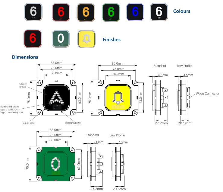
Jumbo Pushbuttons can be supplied loose or incorporated into stations with 1.5mm or 2.5mm stainless steel faceplates, with a vertical pitch of 80mm and horizontal pitch of 90mm i.e the pushbutton body can be rotated through 90 degrees (horizontal version shown above). If pushbuttons are supplied loose, spacers are provided to accommodate the differing faceplate thickness.
